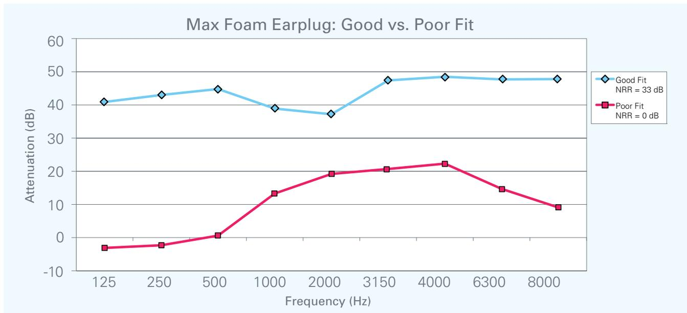
Figure 1. Demonstration of good and bad earplug attenuation across 125-8000 Hz using the Howard Leight® Max® single-use earplug. Test data from Howard Leight Acoustical Laboratory, San Diego, CA.
